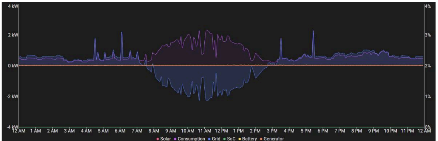
Figure 9: Backwards or swapped CTs with solar power, no battery contribution
